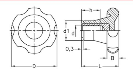
$\begin{array}{ll} B & = 16 \\ D & = 61 \\ d1 & = 25 \\ d \ 6H & = M8 \\ h & = 20 \\ L & = 38 \end{array}$
